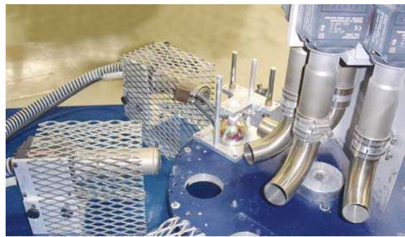
High end hot air systems on an indexing table for producing light bulbs.
